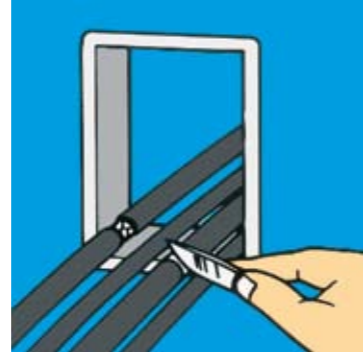
2 Pull cables to final position. Mark cable 30 mm from front edge of frame. Remove cable sheath 5 mm on either side of the line.
