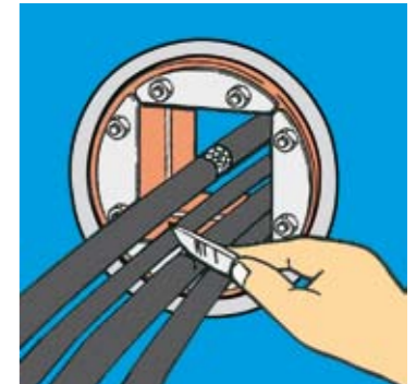
3 Pull the cables to final position. Mark cable 30 mm from front edge of frame. Remove cable sheath 5 mm on either side of the line.
