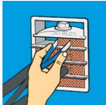
6 Tweezers can be used, if required to aid installation of the last row of blocks.
