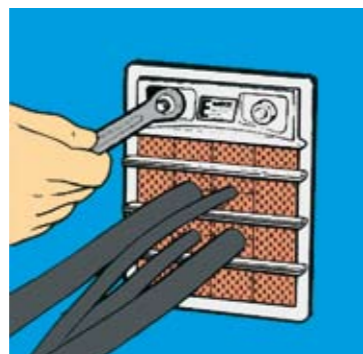
8 Put the endpacking with the tongue around the bolt. Tighten the nuts in the endpacking until approximately 10-12 mm of free threads are visible.
