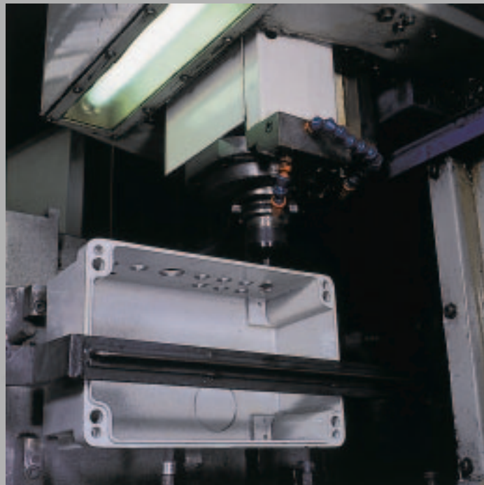
Drilling/threaded an aluminium enclosure
